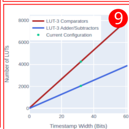
Figure: R2U2 Configuration Explorer web application: 1) C2PO specification input; 2) C2PO options; 3) C2PO output; 4) AST visualization; 5) AST node data; 6) R2U2 instruction; 7) C engine speed and memory calculator; 8) FPGA speed and size calculator; 9) FPGA design size vs maximum timestamp value.
